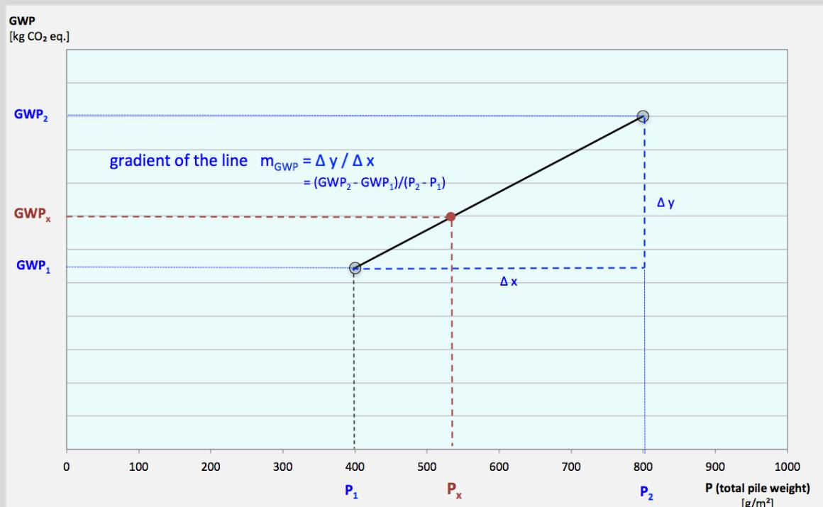
The GWP can be calculated for each product with its individual total pile weight according to the formula
